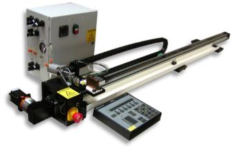
The JNM200 Jacketing and Necking machine gives you control over your critical tubing dimensions. Use the Necking function to precisely control both tube ID and OD. The onboard adjustable temperature controller precisely controls the die temperature for consistent results.
